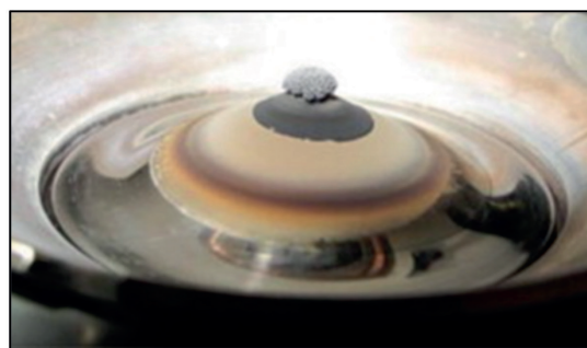
Figure 6: An ICP-MS sampler cone that has been blocked by carbon deposits building up on the tip after extended use of aspirating organic-based samples.
